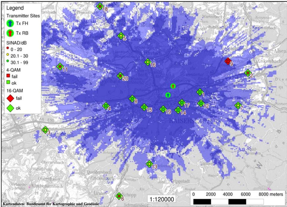
Fig. 2. Predicted vs. measured coverage for DRM+ with TX RB is switched off. Predicted coverage: 4 QAM light blue, 16 QAM dark blue. Assignment of measured coverage see Tab. 3.
