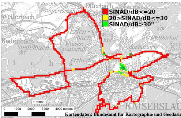
Fig. 6. Measured mobile coverage for FM with TX RB operating at 35 W in the first neighbouring channel (87.7 MHz). Assignment of measured coverage see Tab. 3.
