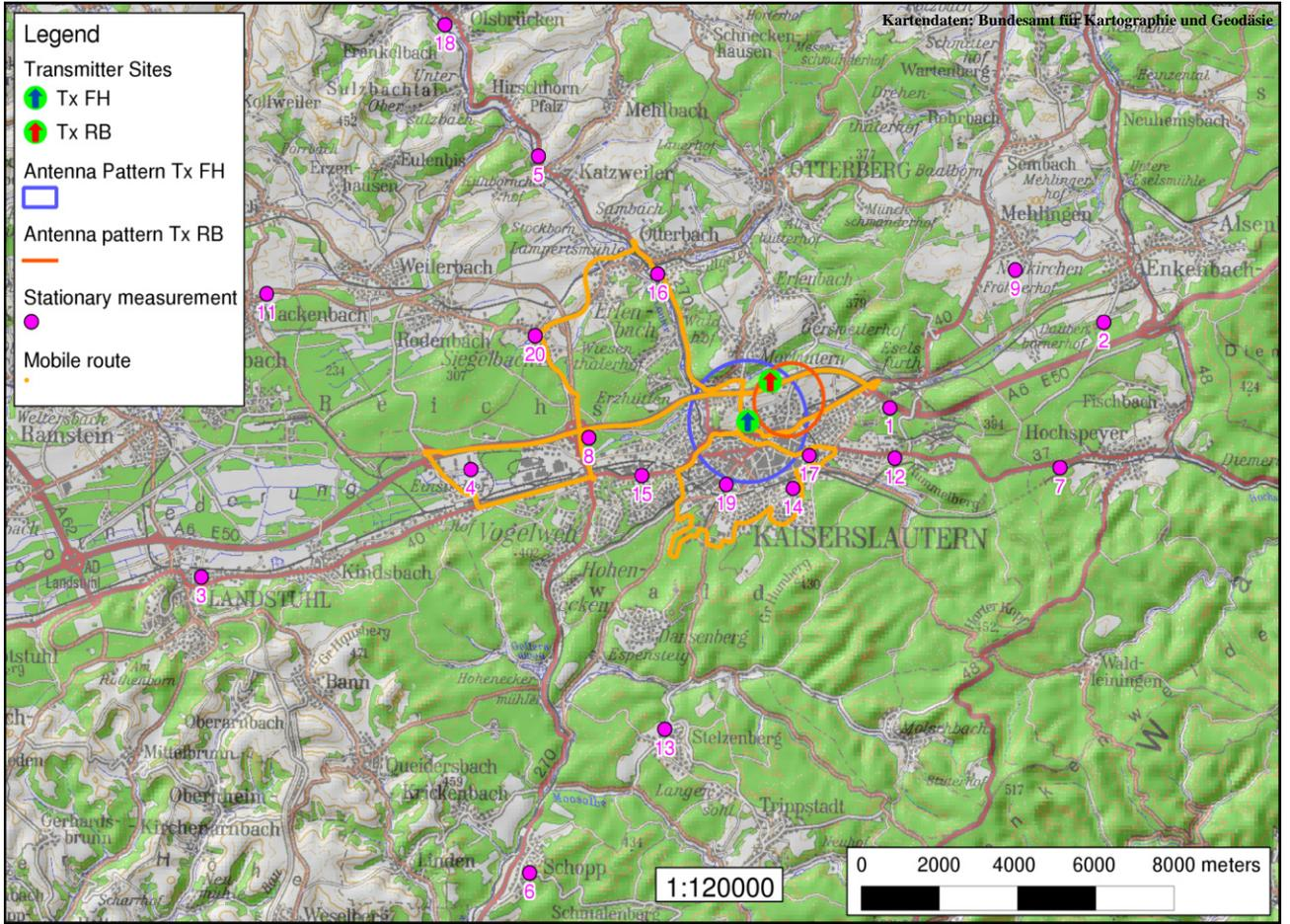
Fig. 1. TX locations, 19 points of stationary measurements, and, mobile measurement route (54 km)
