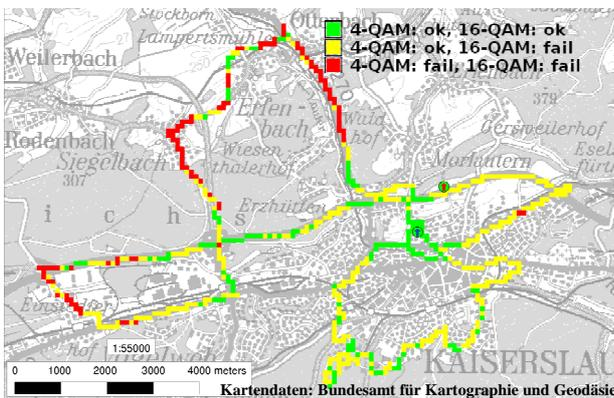
Fig. 7. Measured mobile coverage for DRM+ with TX RB operating at 35 W in the first neighbouring channel (87.7 MHz). Assignment of measured coverage see legend.
