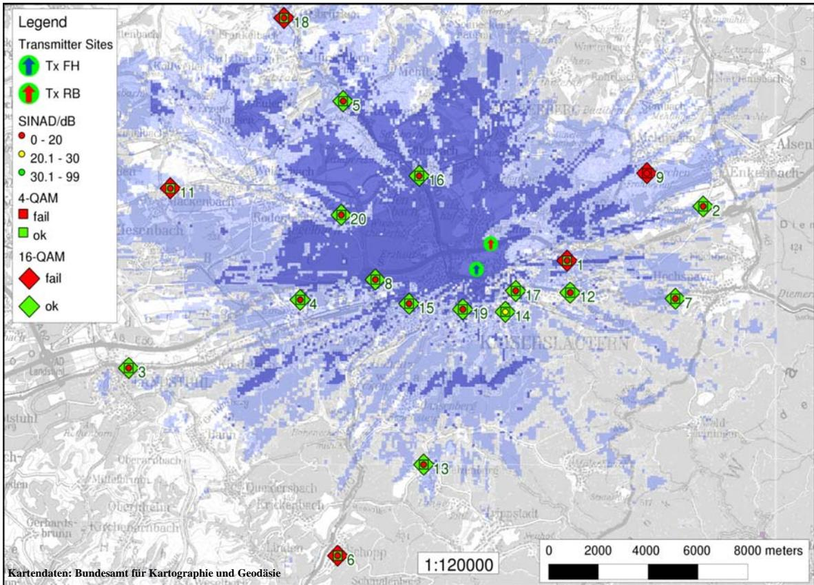
Fig. 3. Predicted vs. measured coverage for DRM+ with TX RB operating at 35 W in the first neighbouring channel (87.7 MHz). Predicted coverage: 4 QAM light blue, 16 QAM dark blue. Assignment of measured coverage see Tab. 3.
