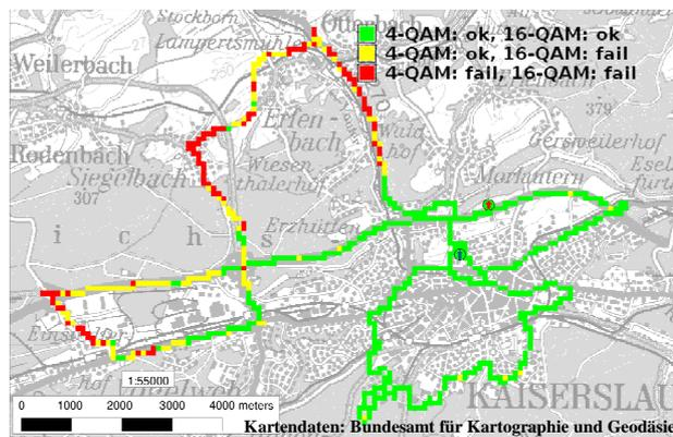
Fig. 5. Measured mobile coverage for DRM+ with TX RB switched off. Assignment of measured coverage see legend.
