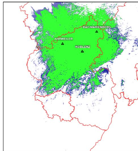
Fig. 5: DRM+ coverage of SFN KOBLENZ
