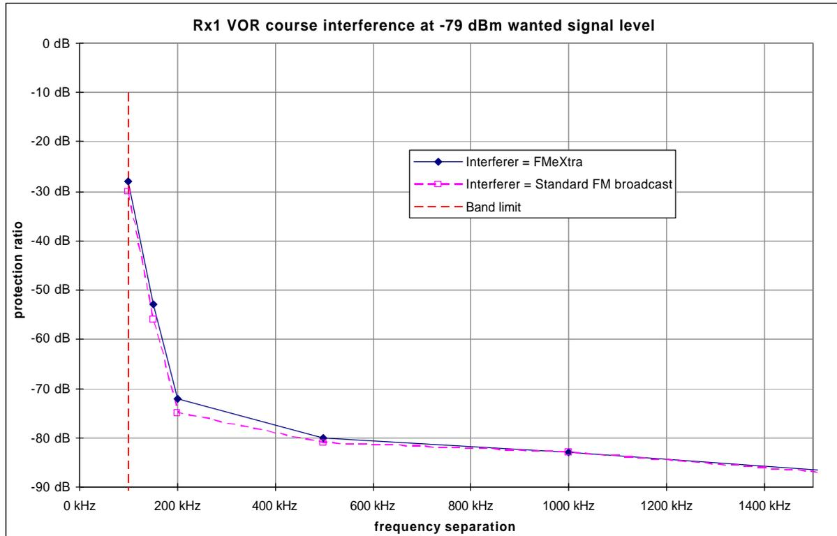
Fig. 7: Protection ratios for VOR interfered by standard FM broadcast and FMeXtra signals
