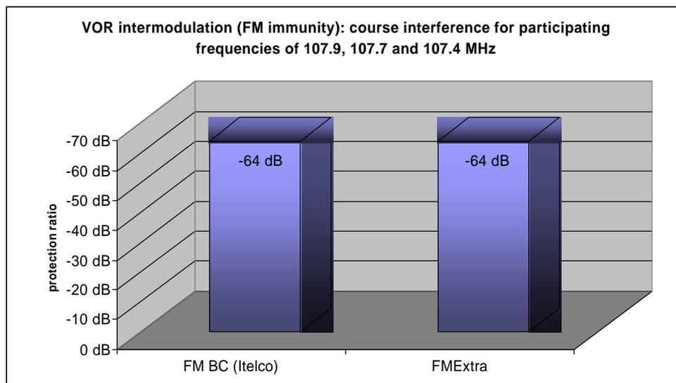
Fig. 10: „FM immunity“ of VOR in the presence of strong analogue and digital broadcast signals
