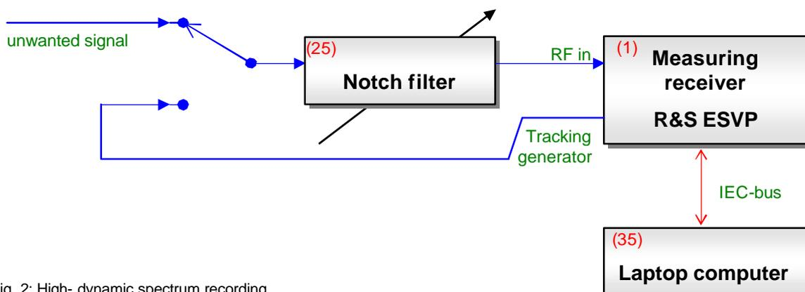
Fig. 2: High- dynamic spectrum recording
