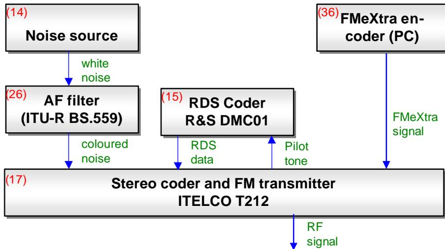
Fig. 4: Block diagram of the unwanted FM broadcast and FMExtra signal generation. Numbers in brackets refer to the measurement equipment list in Annex 1
