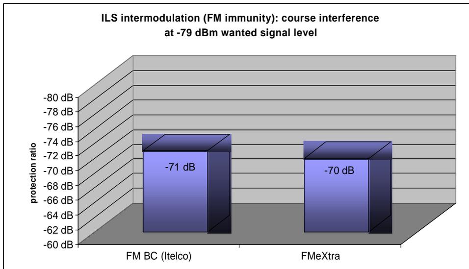
Fig. 11: „FM immunity“ of the ILS localizer in the presence of strong analogue and digital broadcast signals
