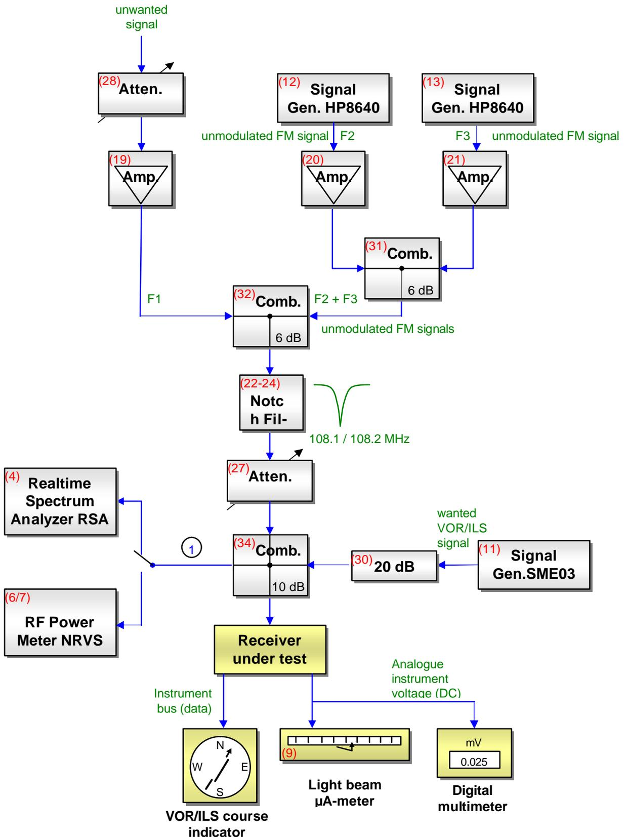
Fig. 9: Setup for FM immunity measurements according to ITU-R IS.1140 Fig. 1a and 1b
