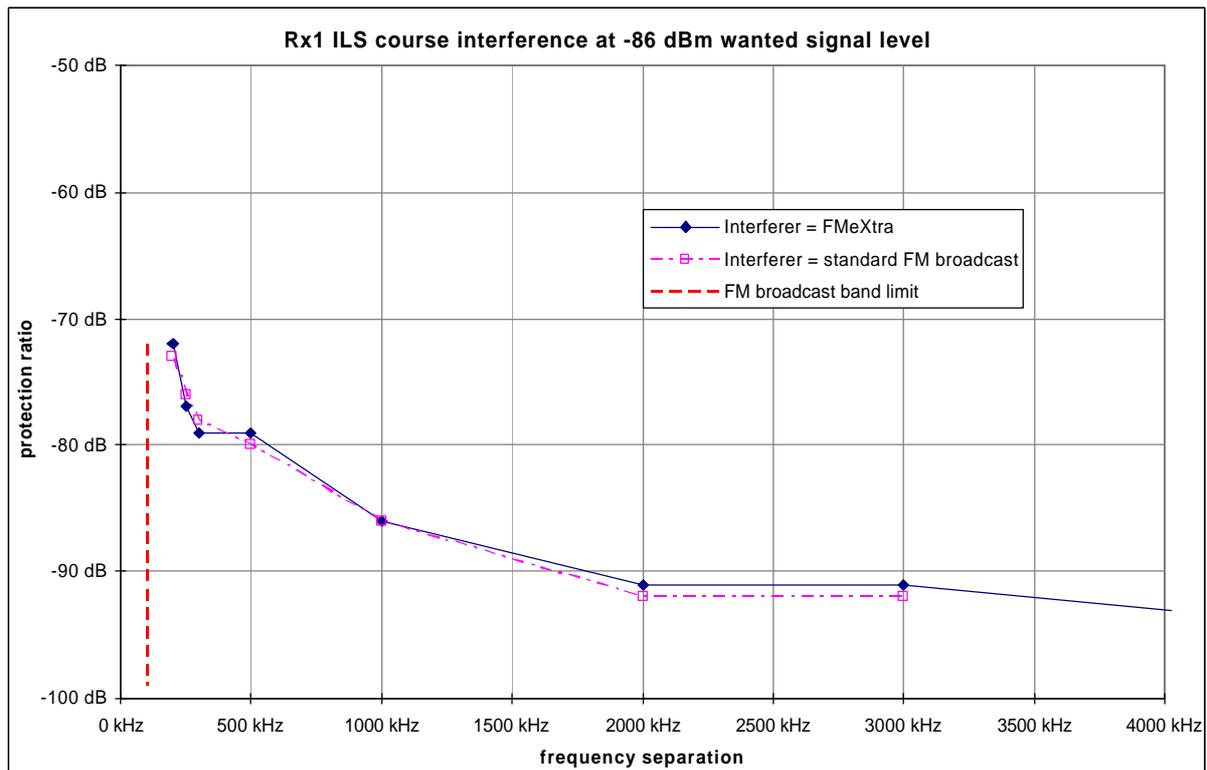
Fig. 8: Protection ratios for ILS interfered by standard FM broadcast and FMExtra signals
