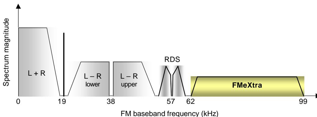
Fig. 3: schematic spectrum of the FM baseband (MPX)
