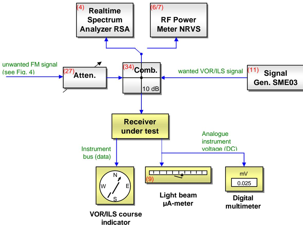
Fig. 6: Setup for protection ratio measurements
